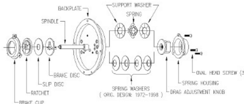
Drag Mechanism - Exploded View
